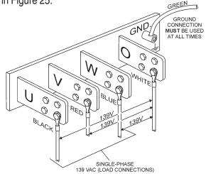
Figure 25. UVWO Terminal Lugs 1Ø-139V Connections
